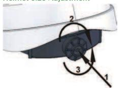
Press the knob (1) to loosen (2) or tighten (3)
